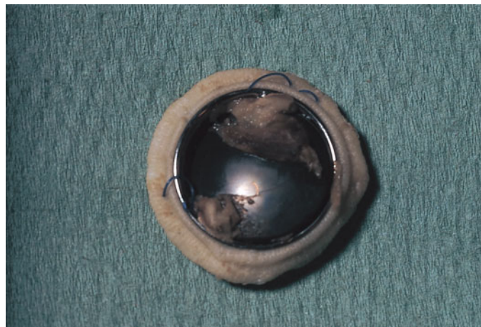
FIGURE 6.74 This plastic flap valve has been surgically removed because it was jammed by formation of thrombus.
